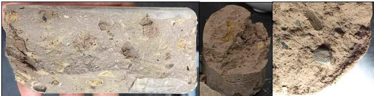
Figure 8. Specimen cross sections showing inclusions
