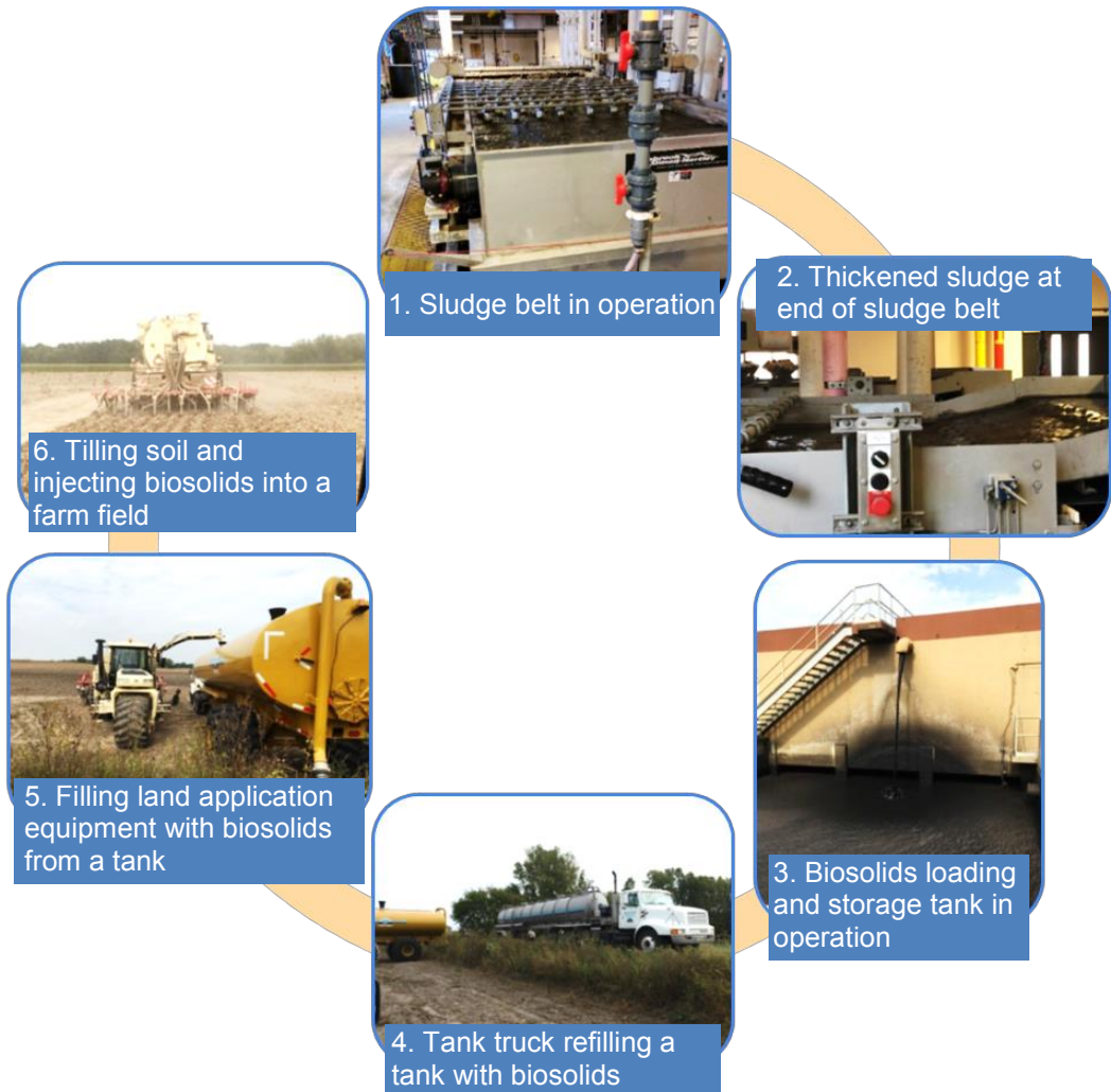
Figure 2: Steps used to create and apply biosolids to the land
