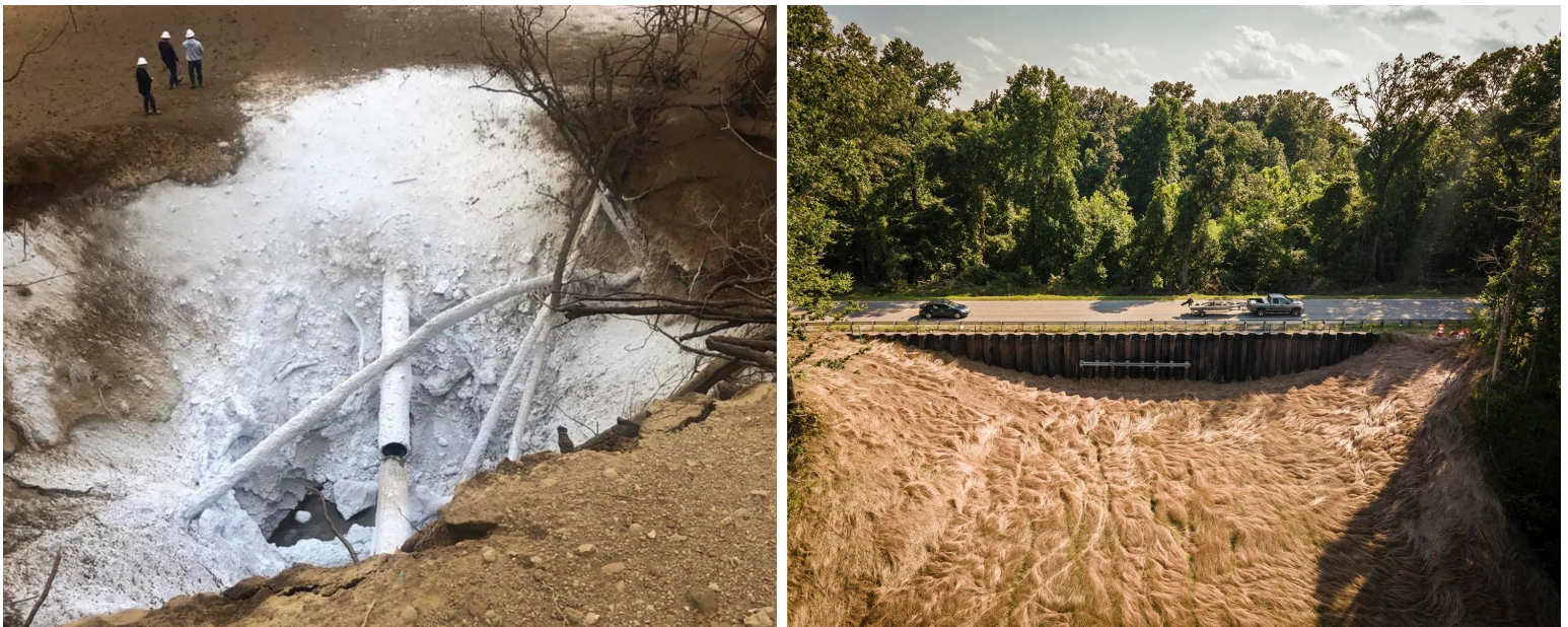
LEFT: The CO2 pipeline rupture. RIGHT: Vehicles pass over the pipeline explosion site in Satartia in July.
