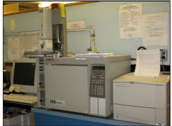
Gas Chromatograph used for analyzing organic chemical contaminants such as PCBs
